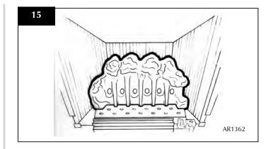
• Place the front coal centrally in the channel at the front of the tray. The relationship between the front coal and the flame baffle is shown, Diagram 16.
